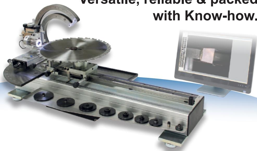
The **Real-Time-Analyser** (= **RTA**) is a system for professional tool analysis coupled with a high-quality optical measuring unit. Due to its modular design it is suitable for analysing the most diverse tools. With the RTA everything that fits under the magnifier can be analysed and it is thus a versatile all-rounder – designed for daily application at the (grinding) machine.
